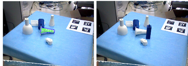
Figure 1. The effectiveness of LINEMOD method with partial foreground occlusions. Left: The target object that is not occluded can be detected in the scene. Right: The target object that is partially occluded cannot be detected in the scene.
