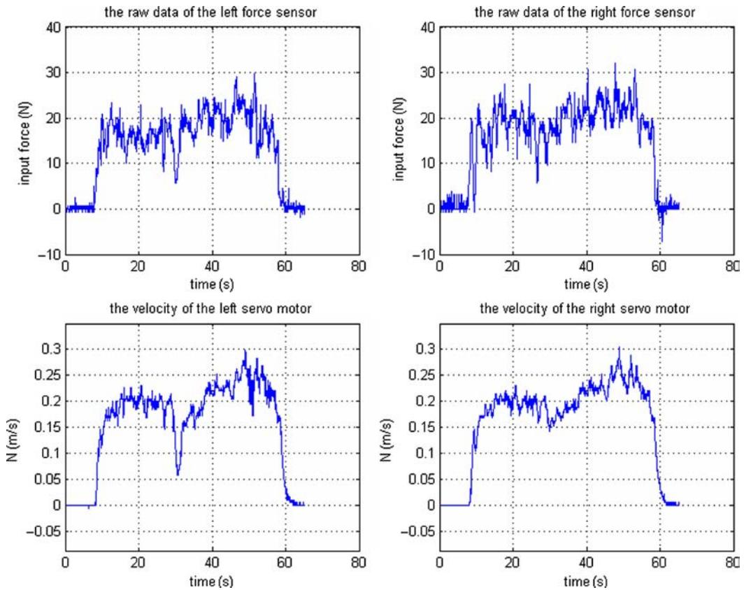
Figure 17 Data of sensors in the force-acceleration mode
