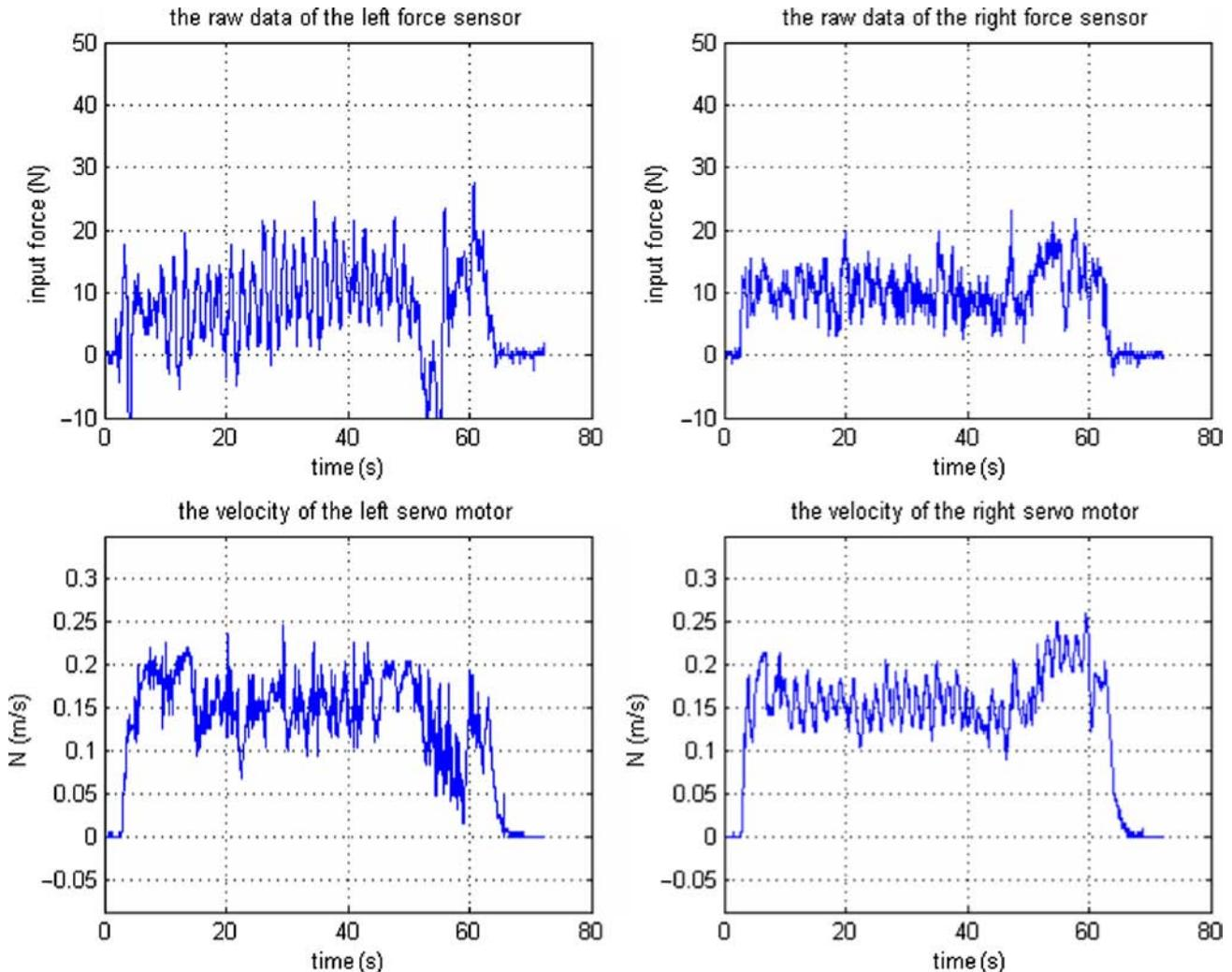
Figure 16 Data of sensors during walking in the force-velocity mode
