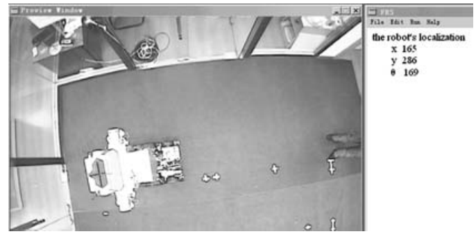
Fig. 5. Localization of the robot by PCS.
