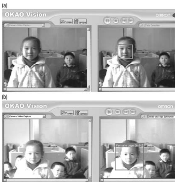
Fig. 4. Face recognition experiment. Processing of (a) face capture (b) face recognition.
