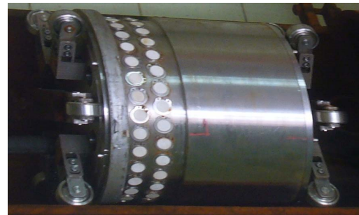
Fig. 2. High resolution ultrasonic on-line inspection tool for \Phi 195 \sim \Phi 297 pipelines
