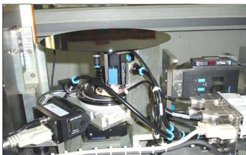
Fig. 4. The proposed wafer prealigner
