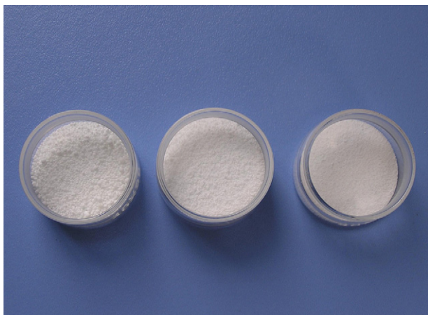
Fig. 14. \text{Li}_4\text{SiO}_4 pebble sample with different diameters.
